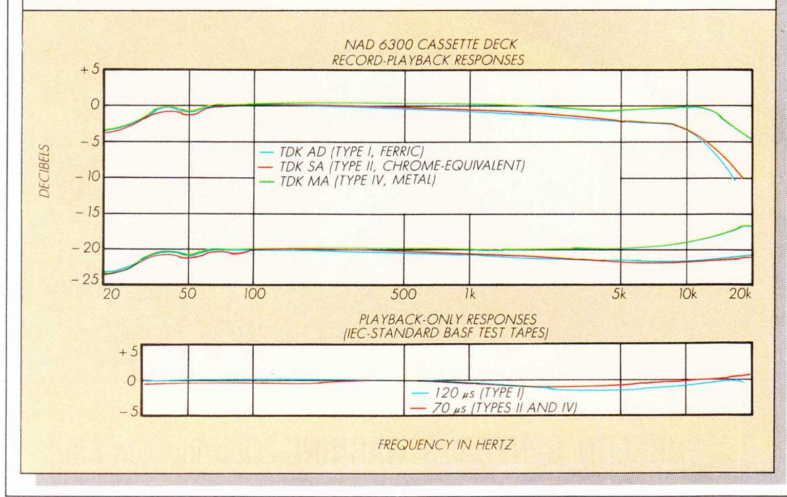
quency level being fed to the record head, and when it senses that the treble saturation point is being reached, it slightly lowers the record bias to give the tape more high-frequency headroom. At normal signal levels the bias level is unaffected and can be set for maximum lowfrequency performance.
